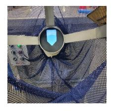
The recovery bag is made of a see thru mesh type material and can be adjusted for use on semi-automatic handguns or rifles. The Brass Catcher can be customized to fit other brands of bullet recovery equipment.
