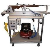
Also, the device is a means of protecting the examiner from the punishing effects of recoil inflicted by the newer generation of high-power weapons.
