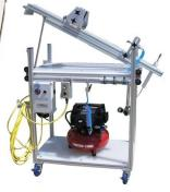
The remote platform is mounted on a custom designed cart that rolls out of the way when not in use. Includes an on-board compressor.
