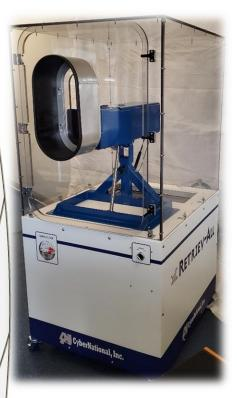
The Retriev-All is principally designed as a Brass and Shell Retrieval System for any weapon ranging from pocket Derringer to 50 CAL. BMG.
